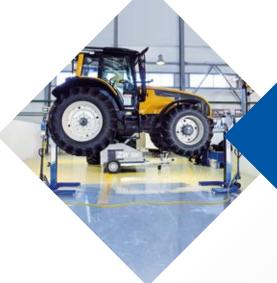
Group and individual column operating modes enable quick and easy replacement of wheel and axle suspensions
